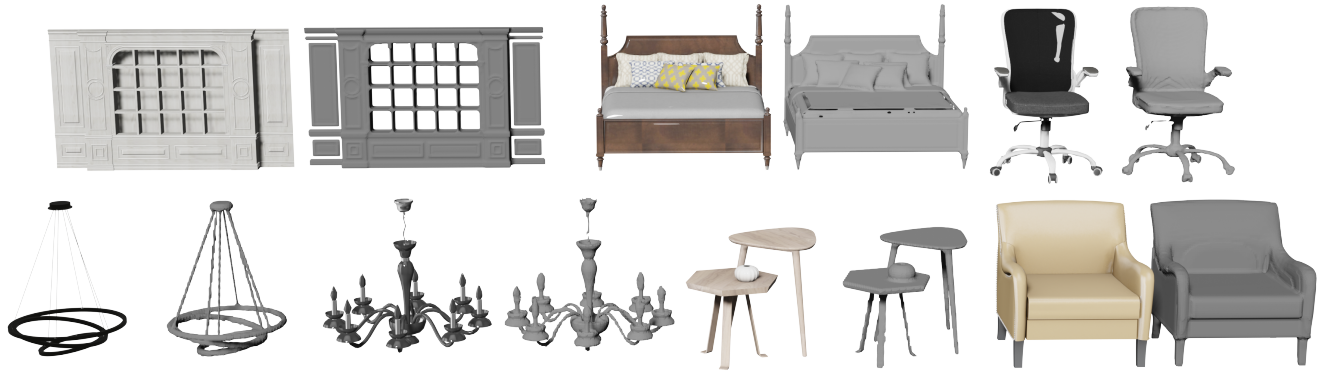
Figure A.1. Original 3D-FUTURE model v.s. re-meshed model. We show examples of re-meshed models. Models on the left model are the original CAD model in 3D-FUTURE, and on the right are the re-meshed models. Despite the perceptual similarity, the re-meshed models fill in the hollow area for collision calculation.
