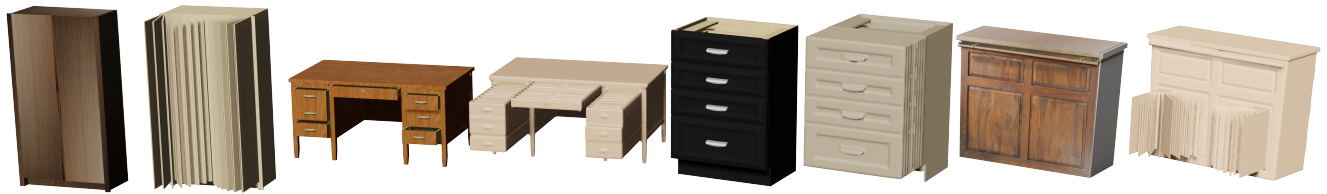
Figure A.2. Original GPartNet model v.s. sequential model. The original CAD models are always in closed status. To simulate the interactive situation, we open the furniture and record the sequential process in an integrated mesh. The left model shows the original furniture, while the right one is the sequential model. We use the sequential model to compute the collision rate of articulated objects.
