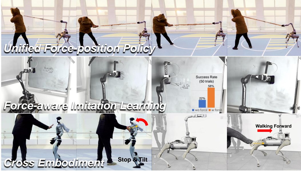
Figure 1: We present a unified force-position policy for legged robots that enables diverse loco-manipulation behaviors, including position tracking, force application, and compliant interactions (top). When used for imitation learning data collection, the policy’s learned internal force estimator provides force-aware demonstrations, improving model performance in contact-rich tasks without external force sensors (middle). Results on quadruped and humanoid robots demonstrate the policy’s versatility and robustness (bottom).
