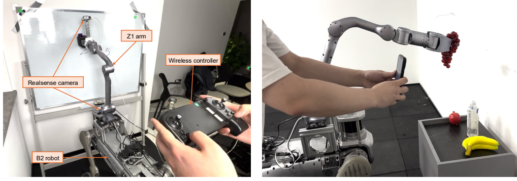
(a) B2-Z1 robot hardware. A Unitree B2 robot with a Z1 arm is teleoperated via a wireless controller, with two RealSense cameras for visual input. (b) iPhone teleoperation. Using the MuJoCo AR app, an iPhone is employed to remotely control the robot for performing manipulation tasks.
