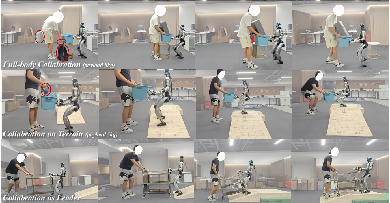
Fig. 1: COLA provides a proprioception-only policy that enables compliant human-humanoid collaboration for carrying diverse objects across various movement patterns. (a) demonstrates horizontal trajectory coordination where the humanoid adapts to human motion patterns. (b) illustrates whole-body coordination during collaborative object-lowering tasks. (c) shows COLA acting as the leader in collaboration with a human to drag a cart up a slope.
